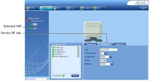
• Confirm that the VCU port is functioning (VAP status LED - top LED in VAP icon associated with this Pod is green).
