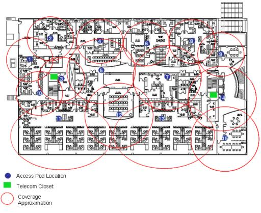
Figure 3-2. Floor Plan Example
