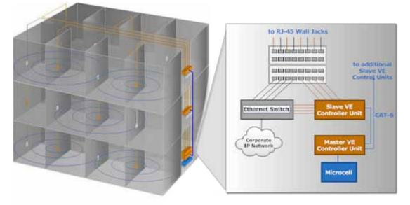
Figure 1-2. Multi-Tier VE Installation
