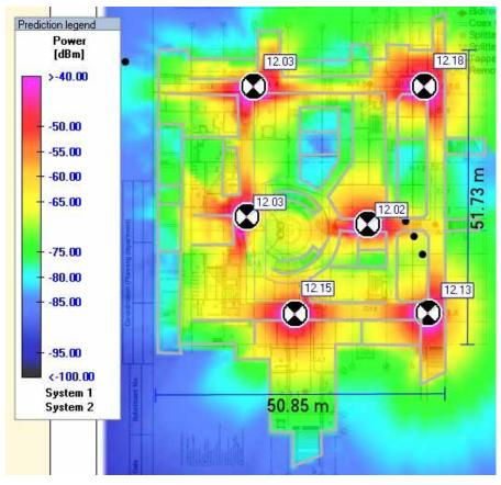
Figure 3-3. Distributed VAPs propagation, 12dBm output power @ 1.8 GHz
