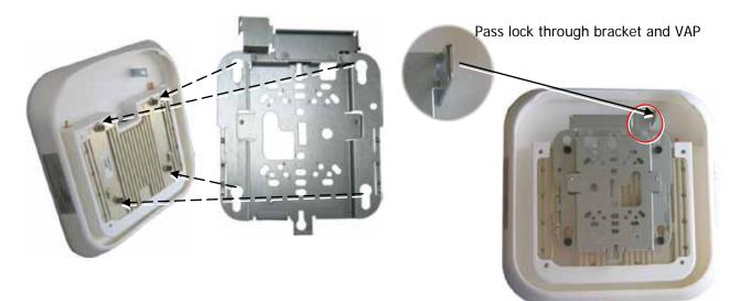
Figure 5-4: Assembling Bracket on to VAP
