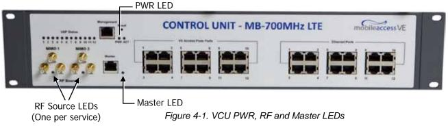
Connect the Slave VCU front panel Master port to the Master VCU VAP port via the patch panel using dedicated STP CAT6 cables. Verify that the Master LED completes initialization (blinking light) and shows a solid green light. The (RF) MIMO LEDs (of both services) should turn OFF.
