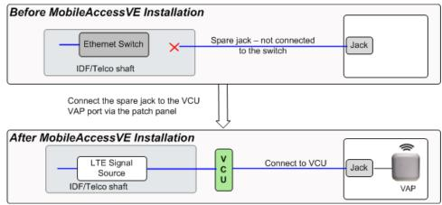
Note: After the Slave VCUs are installed and connected to the correct ports in the patch panels, please proceed with the VAP installation as described in chapter 5. However, it is recommended to complete the VCU provisioning first (See section 4.4) because when installing the VAPs they will instantly provide the wireless service (and the installer will be able to check the coverage).
