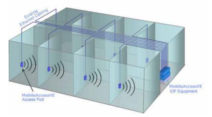
Figure 1-1. Single-Tier VE Installation
