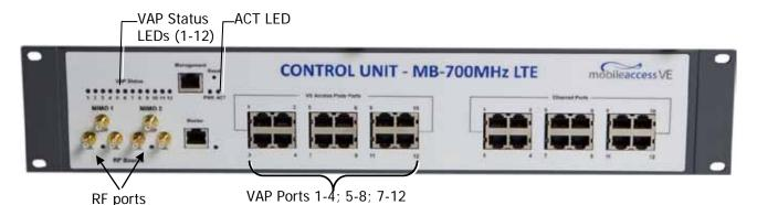
Note 1: After the Slave VCUs are connected (according to section 4.2.2), verify that that the Master VCU **VAP Status** LEDs which correspond to the connected Slave VCUs complete initialization (blinking light) and show a solid green light.
