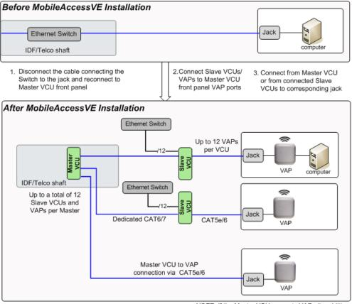
NOTE: If the Master VCU supports VAPs (in addition to Slave VCUs), the relevant Ethernet ports are also connected to an Ethernet switch.
