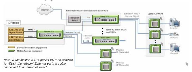
The following figure shows the Multi-tier VE LTE 700 MHz MIMO solution architecture.
