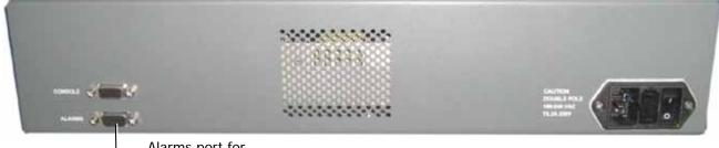
—Alarms port for auxiliary connections
