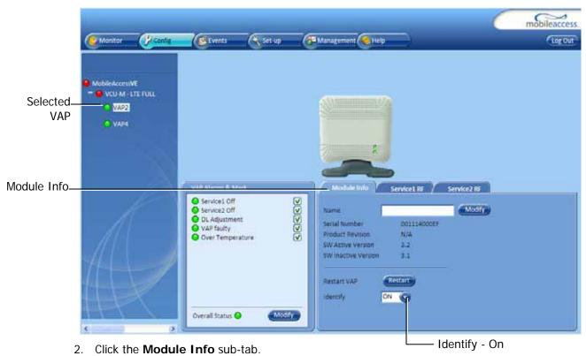
3. Set **Identify** to **ON**. The Activity LED (Blue) on the corresponding Access Pod will start blinking fast. (You will need to physically locate the VAP to see the blinking LED).
