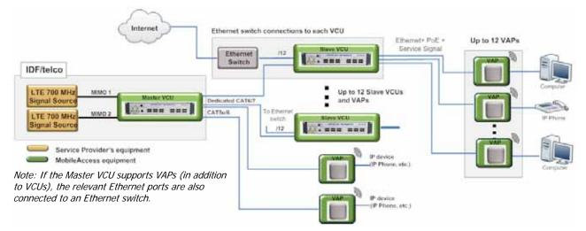
Figure 3-1. VE Multi-Tier Basic Architecture
