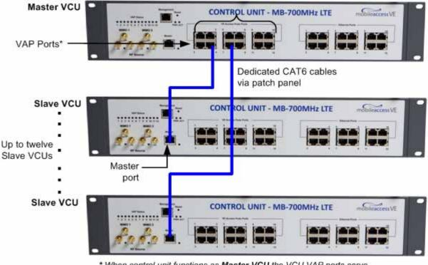
\* When control unit functions as **Master VCU** the VCU VAP ports serve as Slave VCU connection ports
