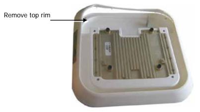
Figure 5-3: Removing Top Rim from Rear of VAP
