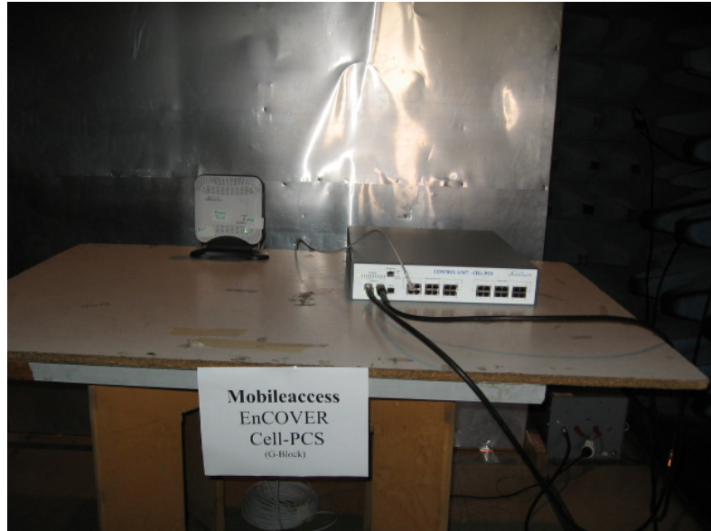
Figure 2. Conducted Emission From AC Mains Test
