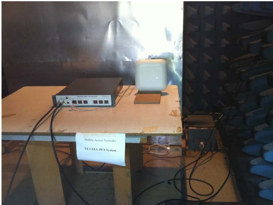
Figure 2. Conducted Emission From AC Mains Test
