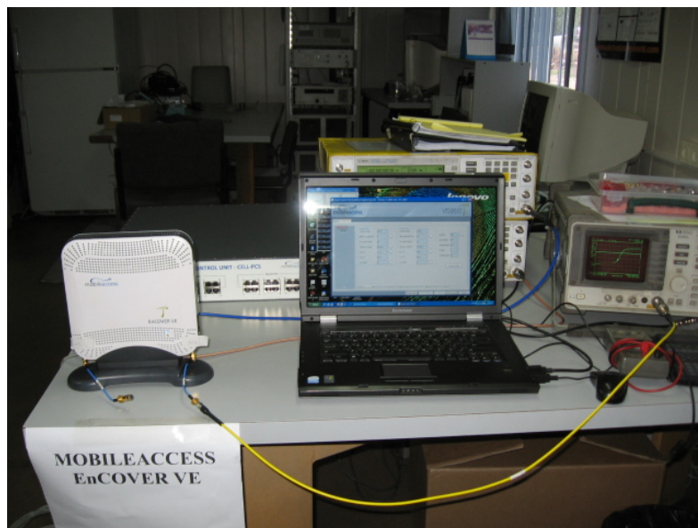
Figure 3. Conducted Emission From Antenna Ports Tests
