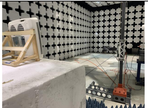
Radiated Emission Test Above 18GHz-50GHz Rear View_2m
