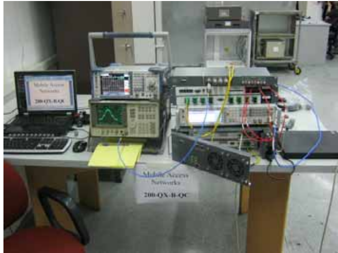
Figure 2. Conducted Emission From Antenna Ports Tests
