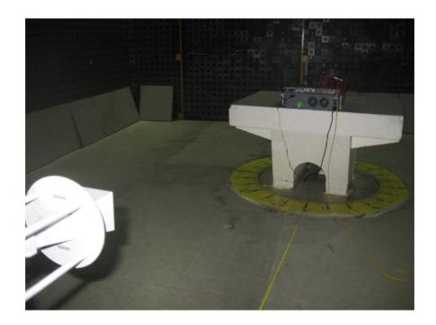
Photograph No.7 Spurious emissions measurement setup at the OATS in 1-18 GHz
