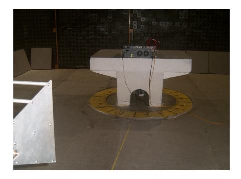
Photograph No.6 Spurious emissions measurement setup in the anechoic chamber in 18-22 GHz
