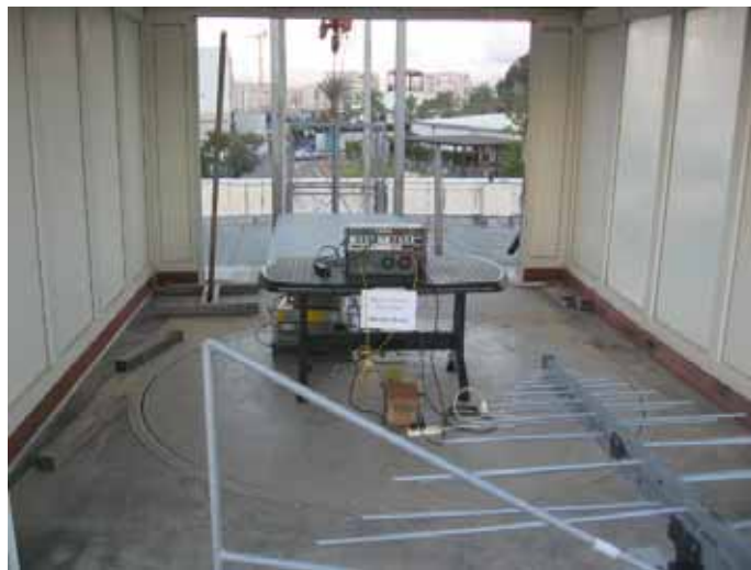
Figure 3. Radiated Emission Test
