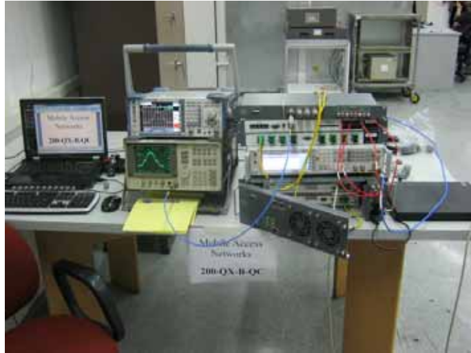
Figure 2. Conducted Emission From Antenna Ports Tests
