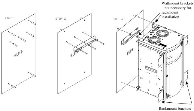
Figure 16: Procedure for Mounting on a Wall
