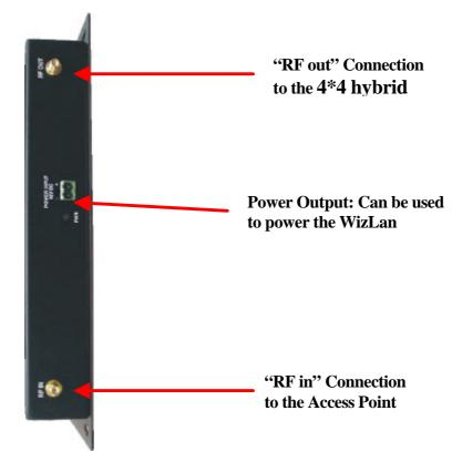
Figure 22: Connector Points on the Auxiliary Modle
