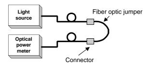
Figure 33: Single Point Test
