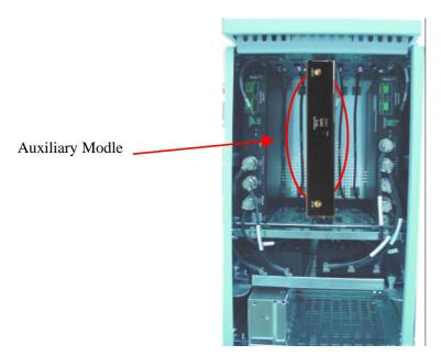
Figure 20: ModuLite<sup>™</sup> MRC Interior with Auxiliary Modle
