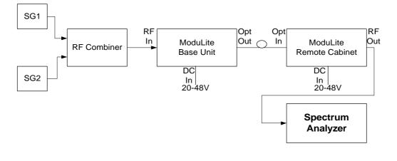
Figure 11: Spectrum Analyzer Setup Test
