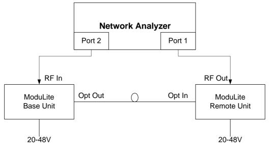
Figure 10: Network Analyzer Setup Test
