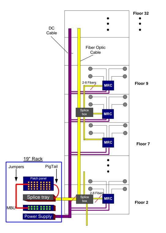
Figure 17: Example - ModuLite<sup>TM</sup> Installation (fiber and coax)
