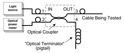
Figure 34: Optical Return Loss Measurement
