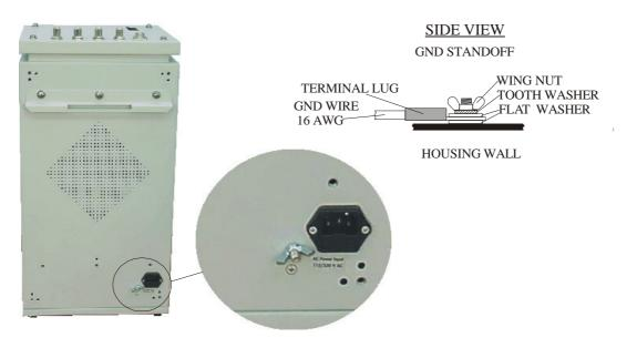
Figure 14: ModuLite<sup>™</sup> GND Standoff Assembly Sequence
