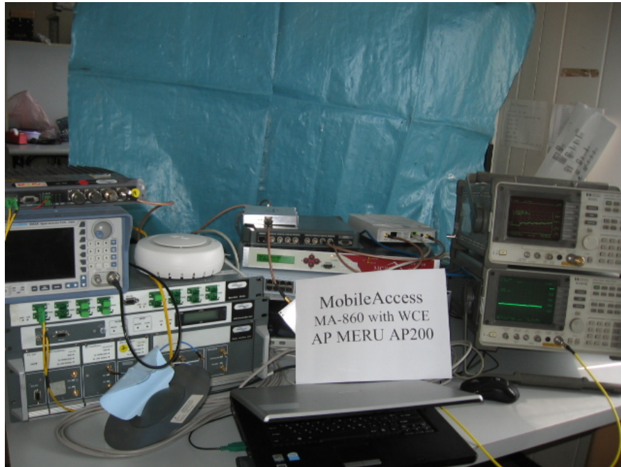
Conducted Tests from Antenna Port With Meru AP200 Access Point
