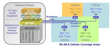
In addition, the MA-860 WLAN solution locates Access Points (APs) in secure telecom closets alongside other LAN internetworking equipment, yielding significant operational benefits:
