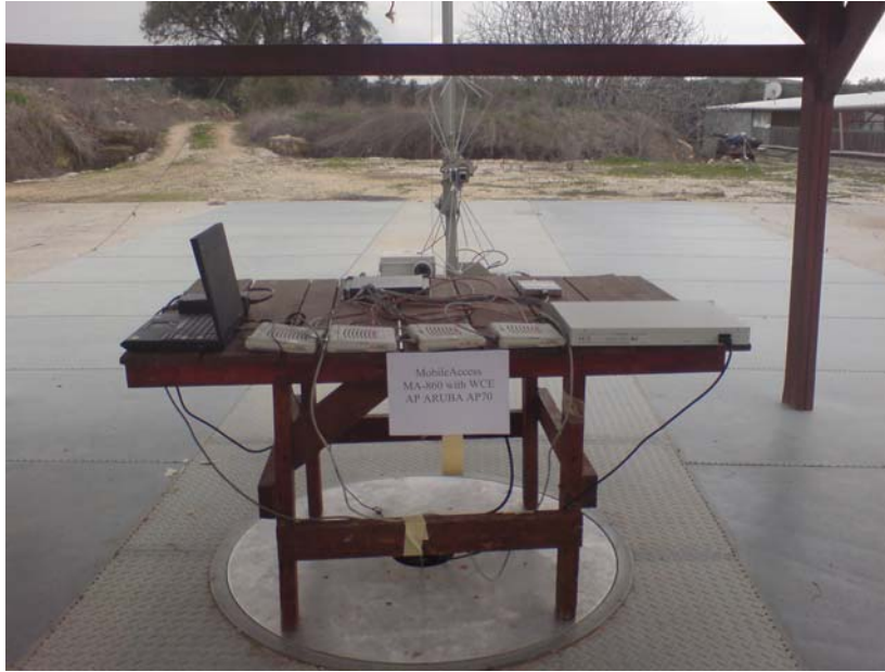
Radiated Emission Test Setup
