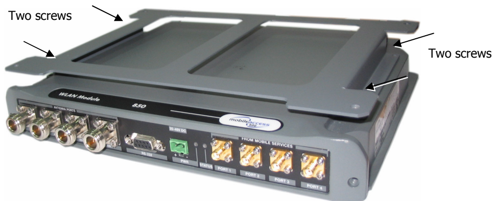
Figure 3-1. MA 850 and Bracket Assembly
