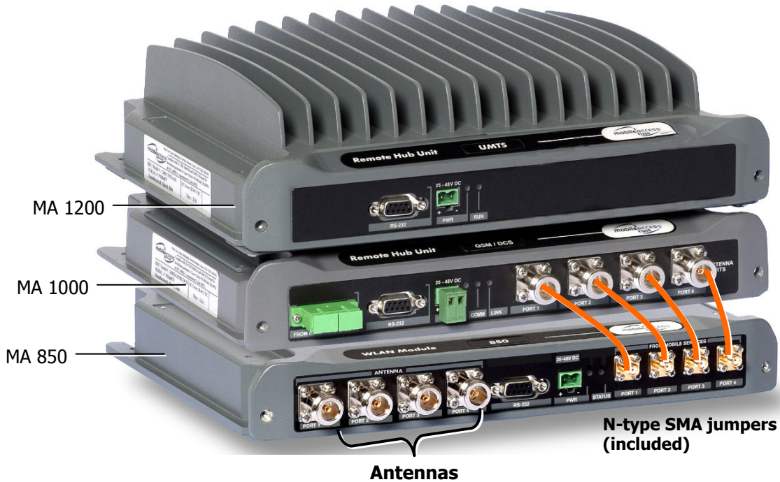
Figure 3-3. Connection of MA 850 and MA 1000 Service Ports
