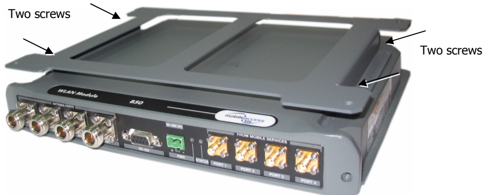
Figure 3-2. MA 850 and Bracket Assembly
