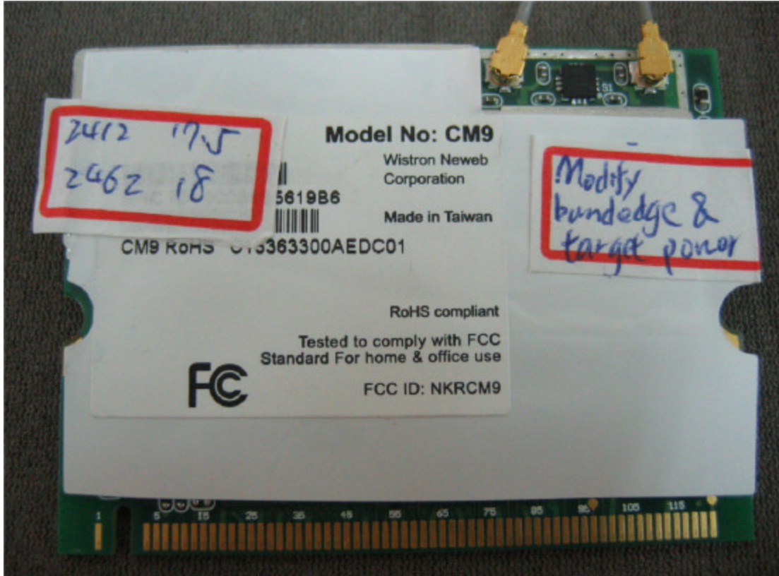
Photograph No.11 Label of Mini PCI card
