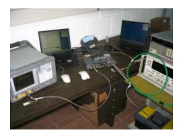
Photograph No.2 Measurements of spurious according to FCC parts 22, 24 at RF antenna connector test setup
