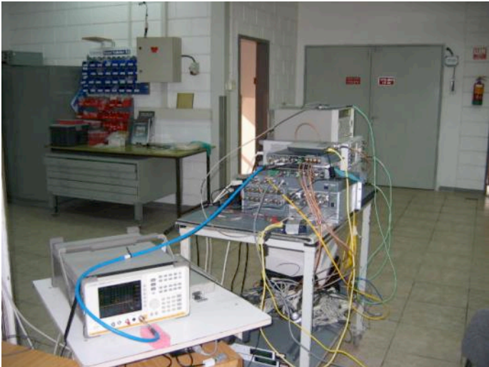
Photograph 1.12.1 Peak spectral power density test setup
