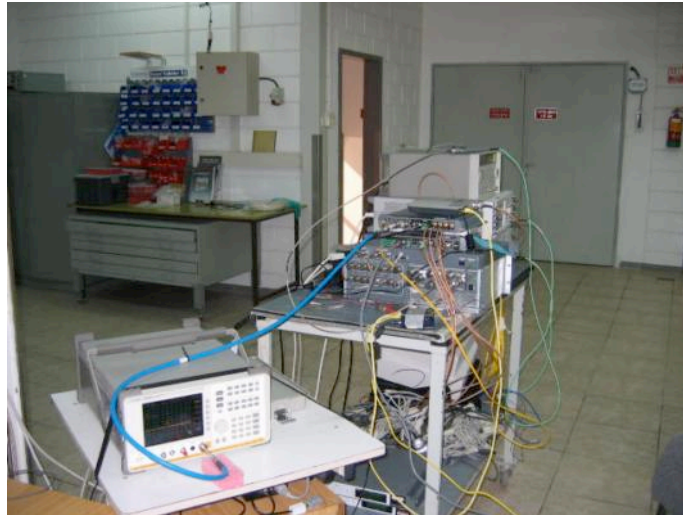
Photograph 1.11.1 Peak spectral power density test setup
