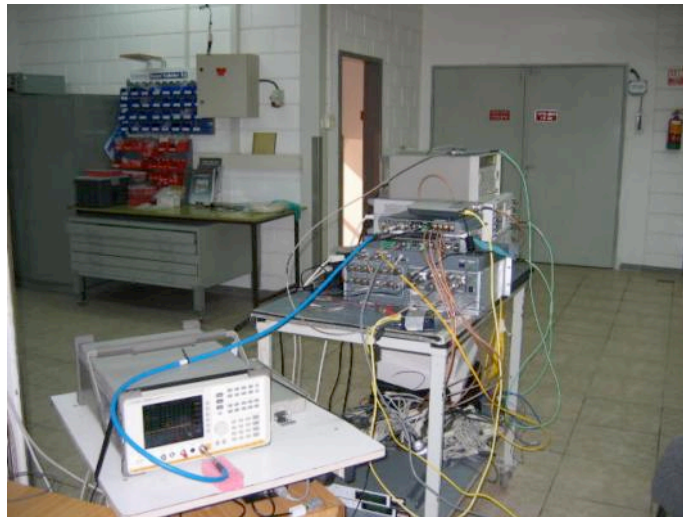
Photograph 1.13.1 Peak spectral power density test setup
