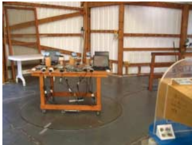
Photograph 7.1.1 Setup for spurious emission field strength measurements above 1000 MHz
