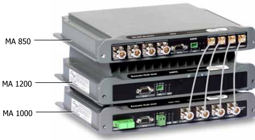
Figure 3-3. Connection of MA 850 and MA 1000 Service Ports
