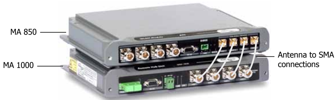
Figure 3-2. Antenna to SMA Connections
