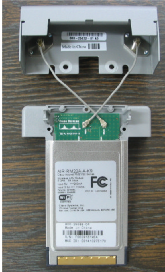
Photograph No.11 Wireless LAN 5.8 GHz module view
