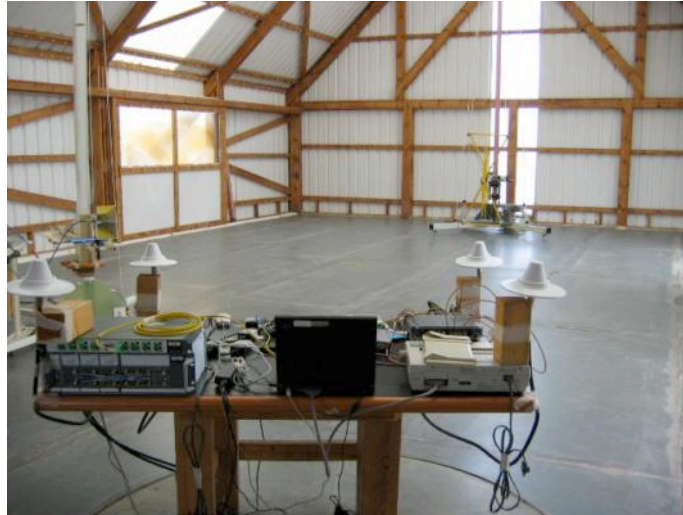
Photograph 2.1.2 Setup for final radiated emission measurements, general view
