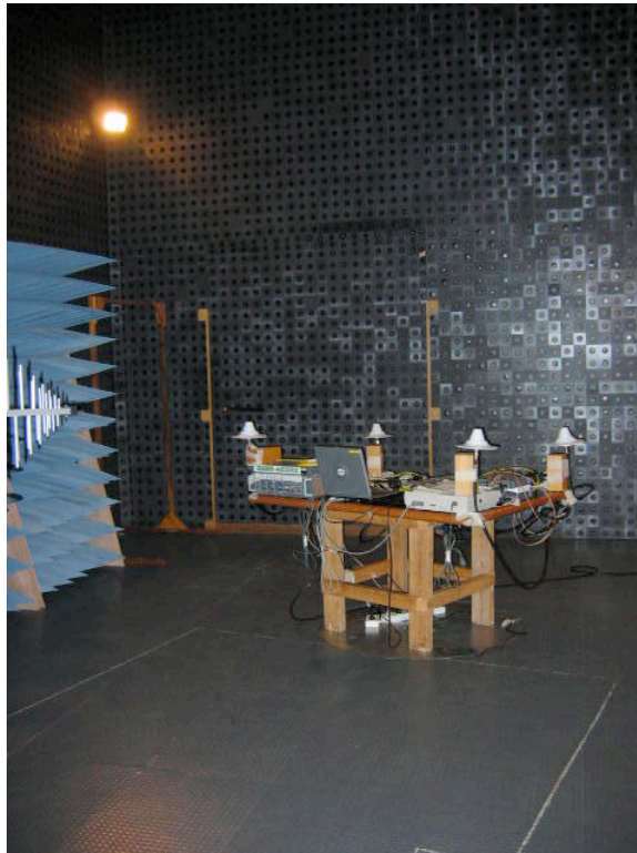
Photograph 2.1.1 Setup for preliminary radiated emission measurements
