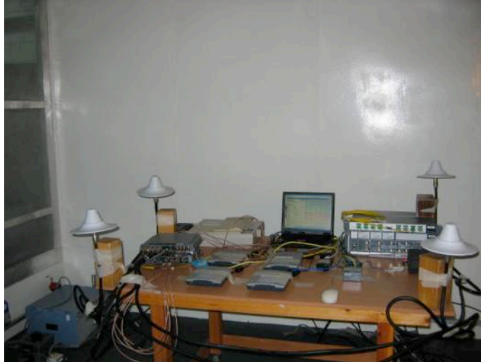
Photograph 1.14.1 Setup for conducted emission measurements
