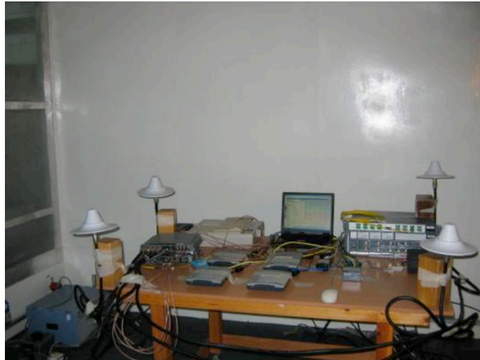
Photograph 1.14.1 Setup for conducted emission measurements
