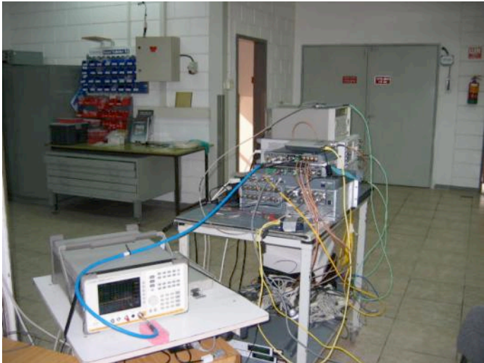
Photograph 1.13.1 Peak spectral power density test setup
