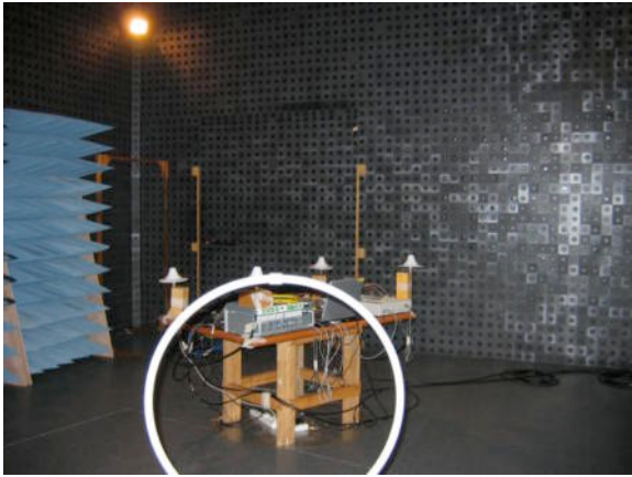
Photograph 1.10.2 Setup for spurious emission field strength measurements from 30 to 1000 MHz
