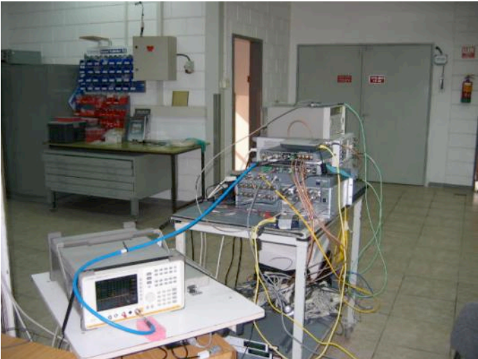
Photograph 1.8.1 Spurious emission test setup
