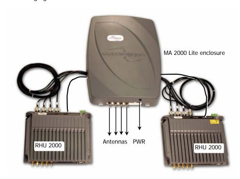
Figure 4-12. 2000 Lite System Coax Connections
