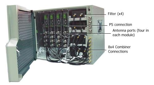
Figure 2-3. RC Open Cabinet with Internal Cabling
