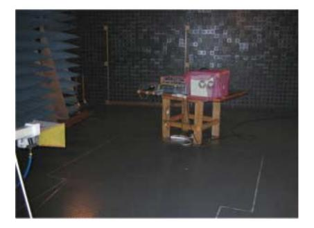
Photograph No.6 Setup for conducted emission measurements at the mains power port
