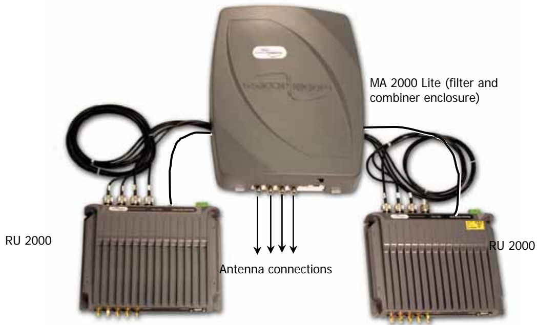
Figure 4-11. 2000 Lite System coax connections
