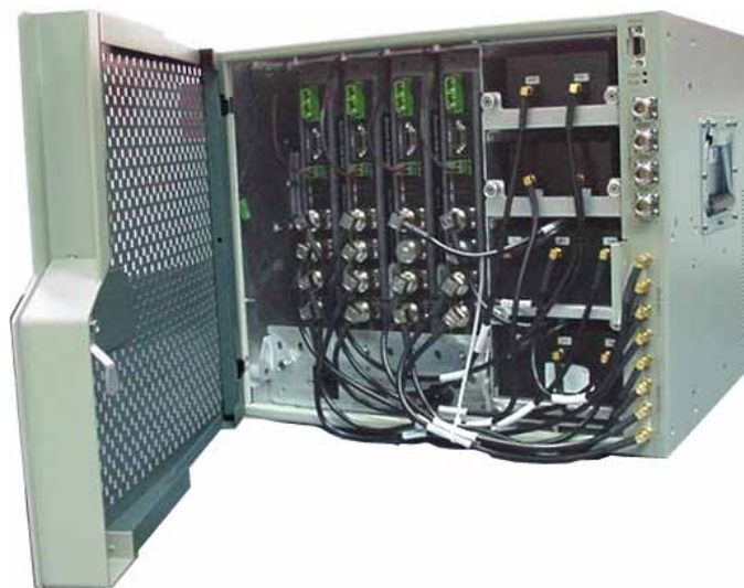
Figure 2-18. RC Open Cabinet with Internal Cabling
