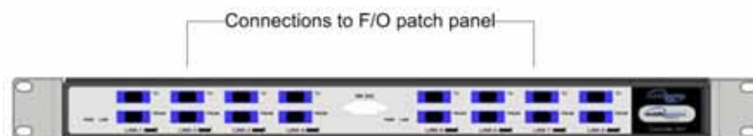
Figure 4-3. BU Front Panel Connections
