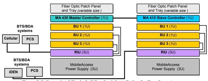
Figure 3-3: Example of Single Building Rack Installation for Two Operators
