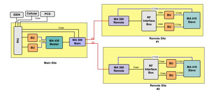
Figure 3-4. Example of Multi-building Topology Communication Room Installation
