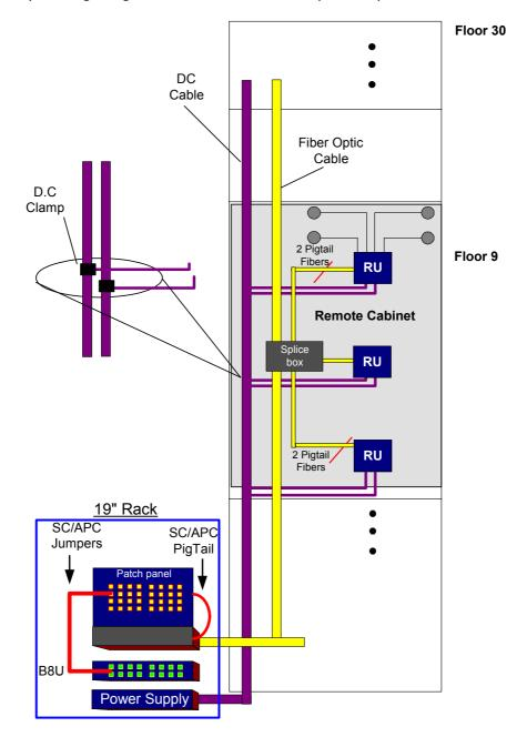
Figure 2-1- Fiber Optic and Power Cables Routing Example
