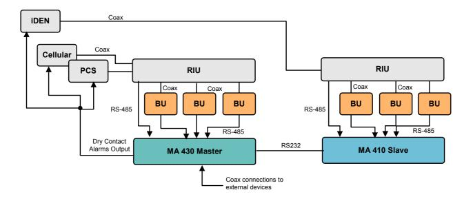
Figure 3-2. Example of Single-building Topology Communication Room Installation
