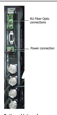
Figure 3-8. RU 2000 Fiber Optic and internal power connections
