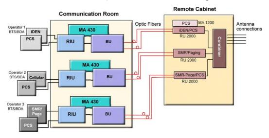
Figure 1-2. Example of a MobileAccess 2000 System
