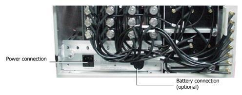
Figure 3-9. Partial View of system illustrating location of power connections
