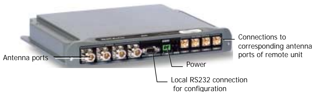
Figure 2-5. MobileAccess 850 Front View
