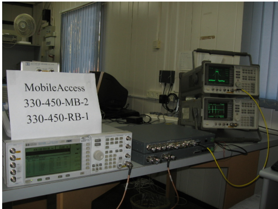
Figure 4. Conducted Emission From Antenna Ports Tests
