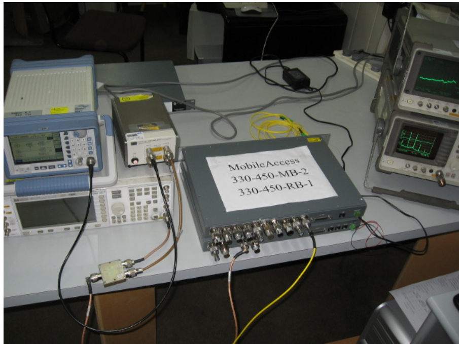
Figure 3. Conducted Emission From Antenna Ports Tests
