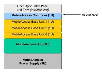
Figure 13: Recommended Order in the Communication Room Rack
