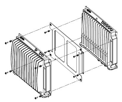
Figure 19. RHU Add-on to 1000 RHU Assembly
