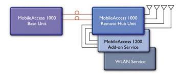
Figure 4. MA 1000/Add-on BU – RHU Plus Add-on Plus WLAN Configuration
