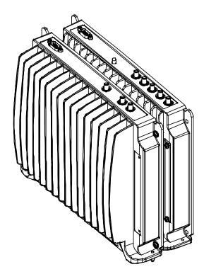
Figure 20. RHU Add-on to 1000 RHU Completed Assembly
