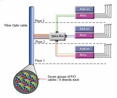
Figure 12. Illustration of Fiber Optic Routing
