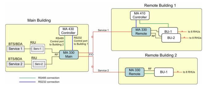
Figure 15: 330 System Installation Examples
