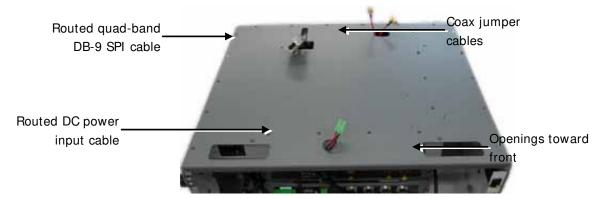
Figure 4-6. TSX Top Cover Openings
