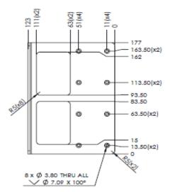
Figure 3-5. Top View of Brackets
