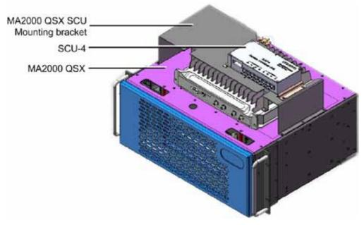
Figure 3-4. SCU-4 Mounted on QSX Unit
