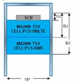
Figure 3-1. Basic MA2000 TSX with SCU-4 Rack Installation Diagram
