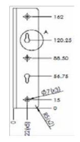
Figure 3-6. Front View of Brackets
