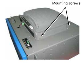
Figure 4-8. AO Unit Mounting Holes – General Location
