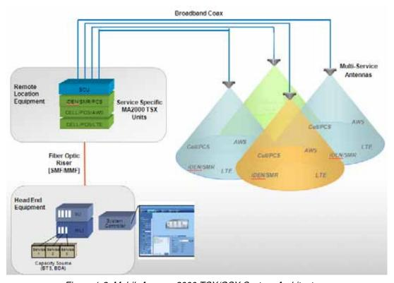
Figure 1-2. MobileAccesss2000 TSX/QSX System Architecture
