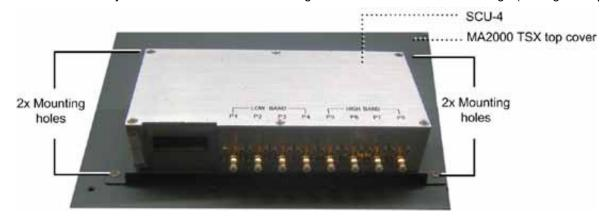
Figure 3-2. SCU-4 Mounted on TSX Unit
