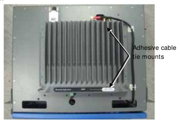
Figure 4-11. Secured High-Band connection
