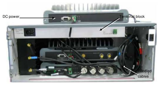
Figure 4-10. Power Connections
