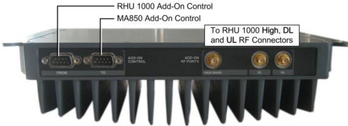
Figure 2. AWS1200 AO Rear Panel
