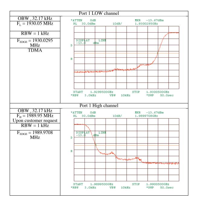
Date 27 May 2004 Test Band edge 15867, Mobile Access 1200 + Mobile Access 1000 Project Humidity 46% Temperature 24 C Air pressure 1014hPa Test equipment521, 1947, 121, 589, 603Assigned bandDownlink:1930 – 1990MHz Uplink:1850 – 1910MHz IP = input power Op = output power $G = gain^{T}$ Mod = input modulation
