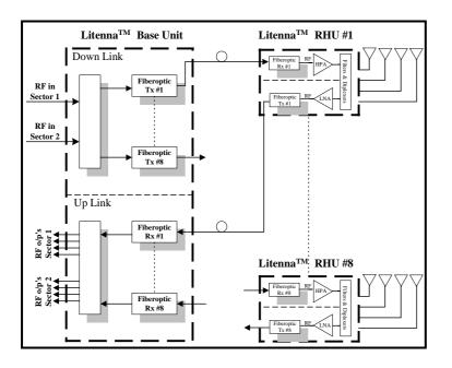
The following is a copy of description of the circuit functions and block diagram of Litenna<sup>™</sup> Model 9A240.
