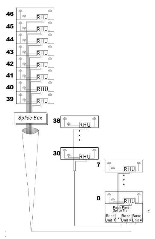
Figure 13 – High Rise Installation
