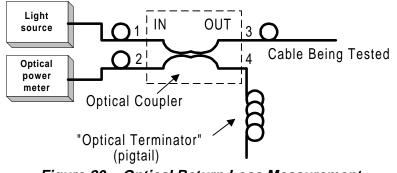
Figure 20 – Optical Return Loss Measurement
