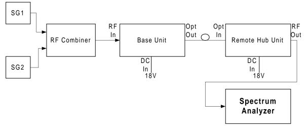
Figure 10 – Spectrum Analyzer Setup Test
