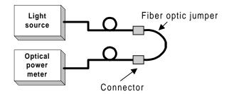
Figure 19 – Single Point Test
