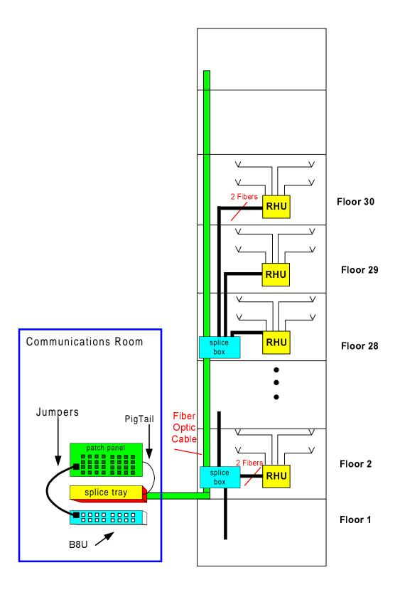
Figure 12 – Example: Fiber Installation
