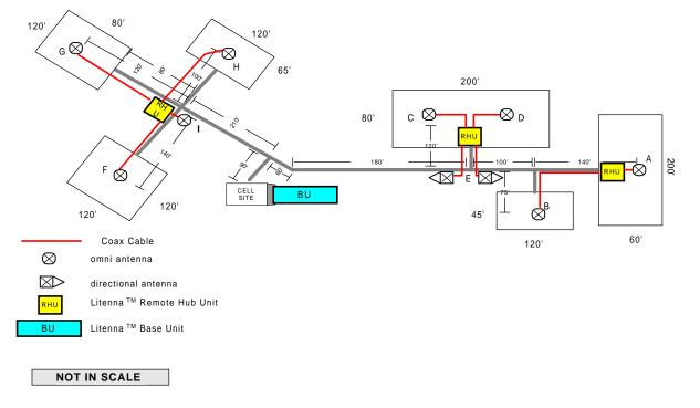
Figure 14 – Horizontal Layout Installation
