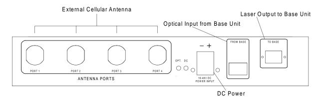
Figure 8 - Remote Hub Unit Front Panel
