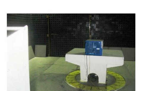
Photograph No.5 Spurious emissions measurement setup in the anechoic chamber in 1-18 GHz
