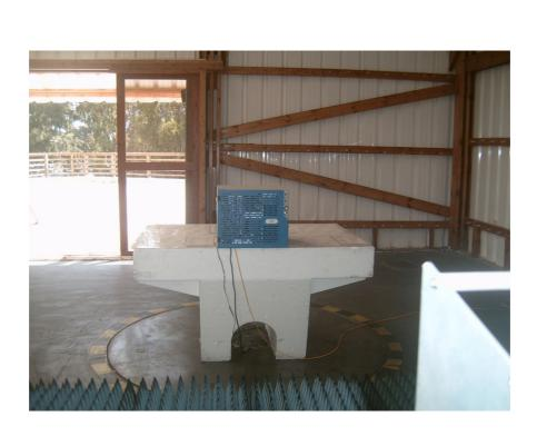
Photograph No.7 Spurious emissions measurement setup at the OATS in 1-18 GHz
