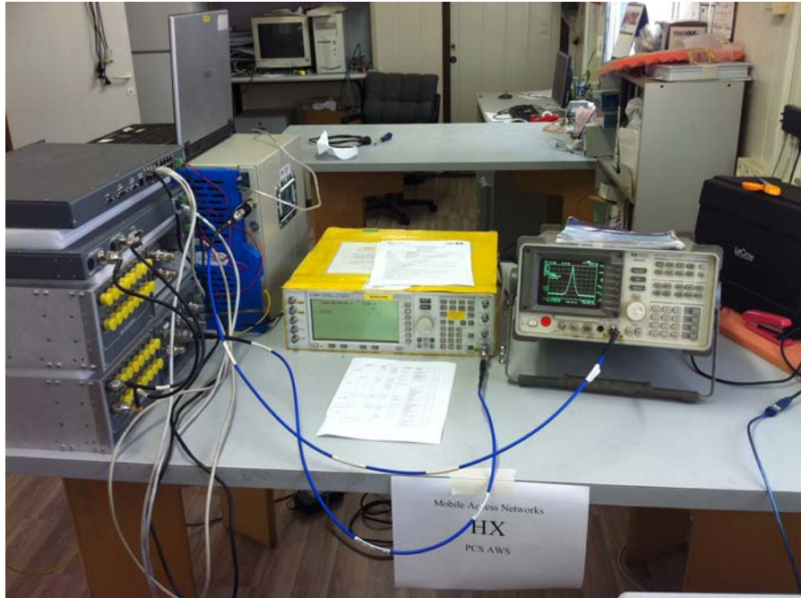
Figure 2. Conducted Emission From Antenna Ports Tests
