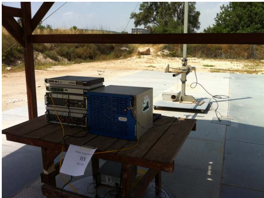
Figure 3. Radiated Emission Test
