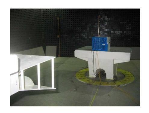
Photograph No.5 Spurious emissions measurement setup in the anechoic chamber in 1-18 GHz
