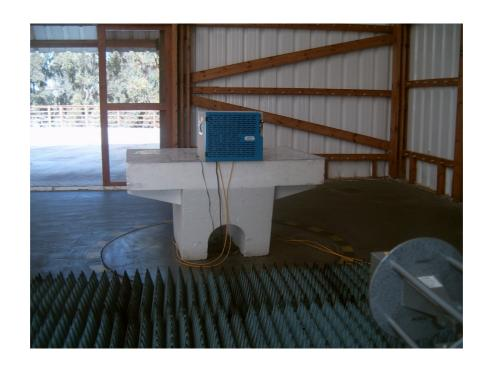
Photograph No.8 Spurious emissions measurement setup at the OATS in 18-22 GHz
