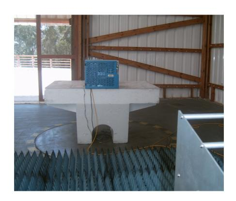
Photograph No.7 Spurious emissions measurement setup at the OATS in 1-18 GHz
