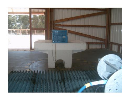
Photograph No.8 Spurious emissions measurement setup at the OATS in 18-22 GHz
