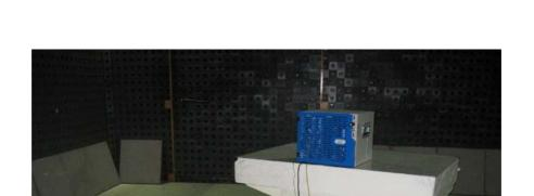
Photograph No.6 Spurious emissions measurement setup in the anechoic chamber in 18-22 GHz
