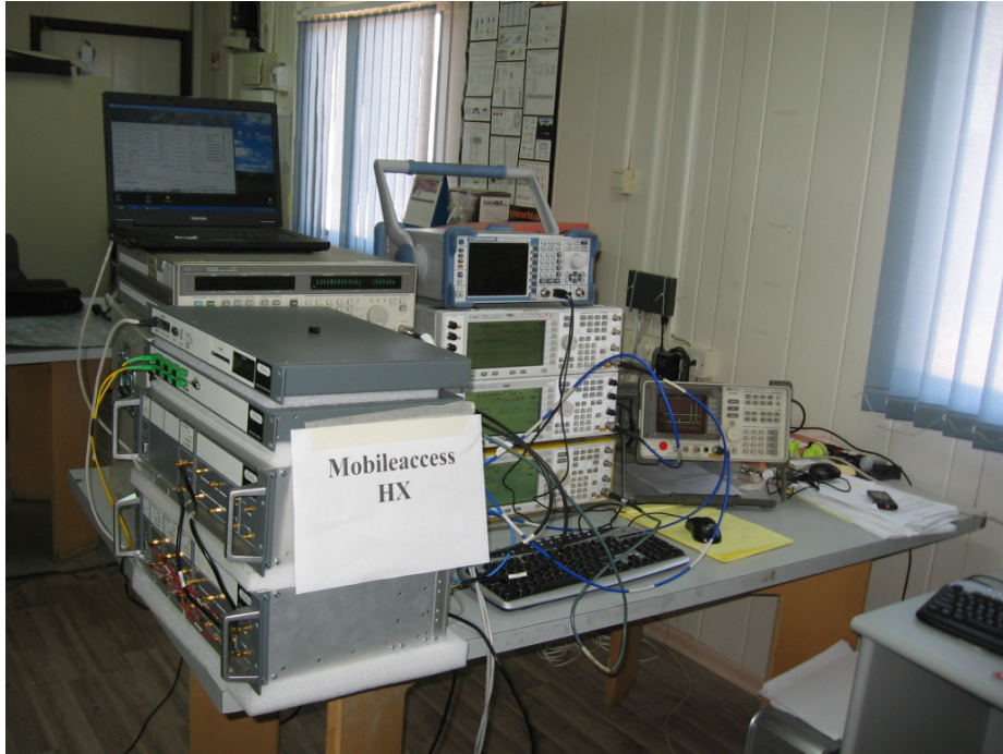
Figure 2. Conducted Emission From Antenna Port Tests
