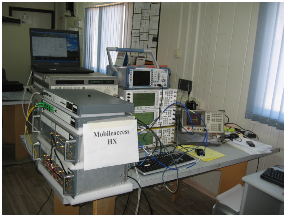
Figure 3. Conducted Emission From Antenna Ports Tests
