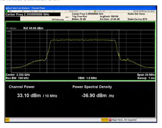
Port1 / LTE 10 MHz / 2 355 MHz / 16QAM
