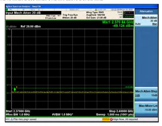
Port1 / LTE 10 MHz / 2 355 MHz / 64QAM / 2 320.0 MHz ~ 2345.0 MHz
