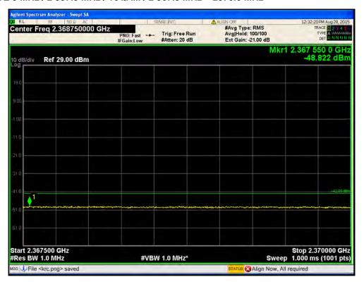
Port1 / LTE 5 MHz / 2 357.5 MHz / 16QAM / above 2 370.0 MHz
