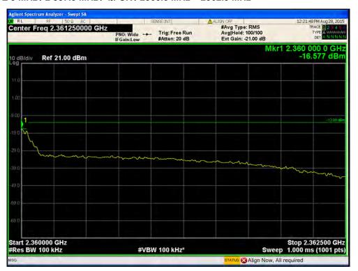
Port1 / LTE 5 MHz / 2 357.5 MHz / QPSK / 2 362.5 MHz ~ 2365.0 MHz
