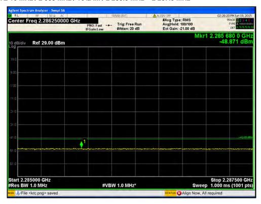
Port1 / LTE 10 MHz / 2 355 MHz / 16QAM / below 2 285.0 MHz
