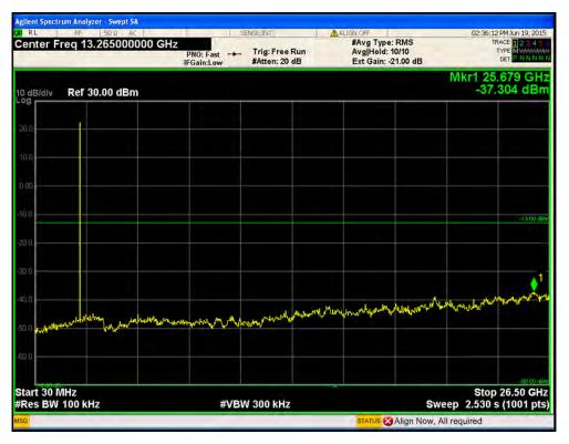
Port1 / LTE 10 MHz / 2 355 MHz / 16QAM / 30 MHz ~ 26.5 GHz
