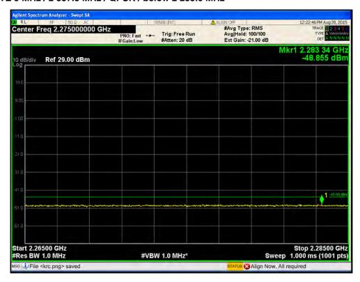
Port1 / LTE 5 MHz / 2 357.5 MHz / 16QAM / 2360.0 MHz ~ 2362.5 MHz
