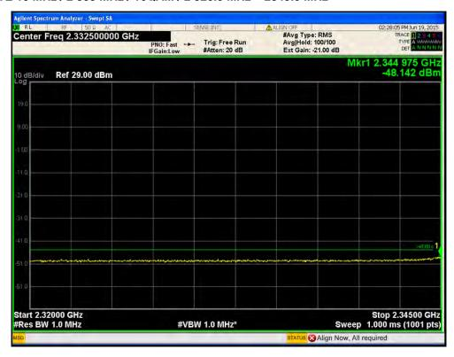
Port1 / LTE 10 MHz / 2 355 MHz / 16QAM / 2 305.0 MHz ~ 2 320.0 MHz
