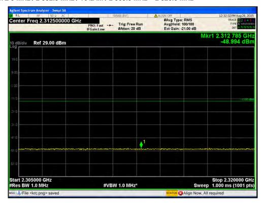
Port1 / LTE 5 MHz / 2 352.5 MHz / 16QAM / 2 300.0 MHz ~ 2305.0 MHz
