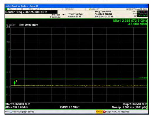
Port1 / LTE 5 MHz / 2 357.5 MHz / 64QAM / 2 367.5 MHz ~ 2370.0 MHz
