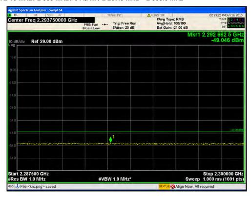
Port1 / LTE 10 MHz / 2 355 MHz / 64QAM / 2 285.0 MHz ~ 2 287.5 MHz
