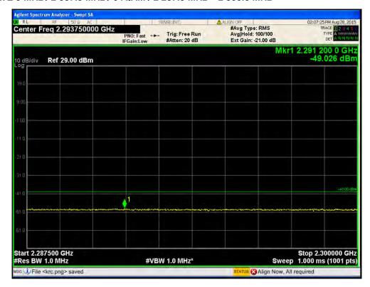
Port1 / LTE 5 MHz / 2 357.5 MHz / 64QAM / 2 285.0 MHz ~ 2 287.5 MHz
