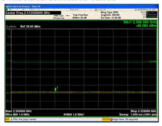
Port1 / LTE 10 MHz / 2 355 MHz / QPSK / 2 300.0 MHz ~ 2305.0 MHz
