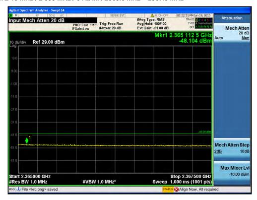
Port1 / LTE 10 MHz / 2 355 MHz / 64QAM / 2 367.5 MHz ~ 2370.0 MHz
