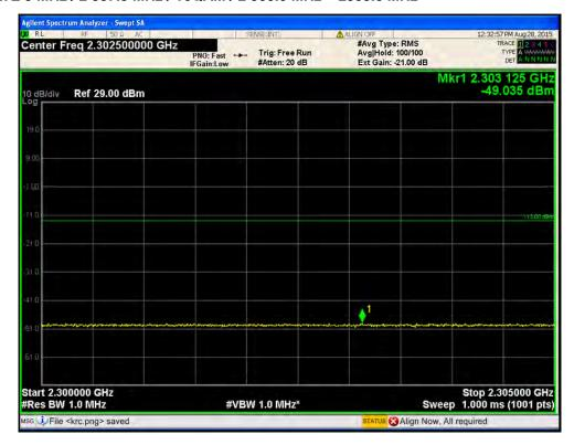
Port1 / LTE 5 MHz / 2 357.5 MHz / 16QAM / 2 287.5 MHz ~ 2 300.0 MHz
