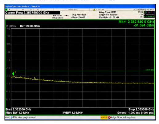
Port1 / LTE 5 MHz / 2 357.5 MHz / 16QAM / 2365.0 MHz ~ 2367.5 MHz
