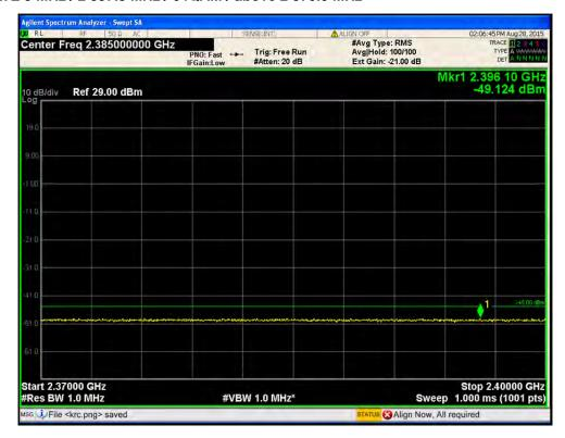
Port1 / LTE 5 MHz / 2 357.5 MHz / 64QAM / 2 320.0 MHz ~ 2345.0 MHz
