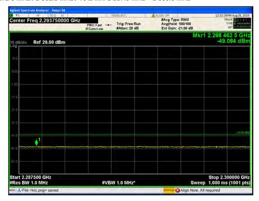
Port1 / LTE 5 MHz / 2 352.5 MHz / 16QAM / 2 285.0 MHz ~ 2 287.5 MHz
