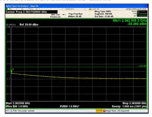
Port1 / LTE 5 MHz / 2 352.5 MHz / 64QAM / 2365.0 MHz ~ 2367.5 MHz
