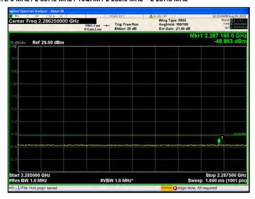
Port1 / LTE 5 MHz / 2 357.5 MHz / 16QAM / below 2 285.0 MHz
