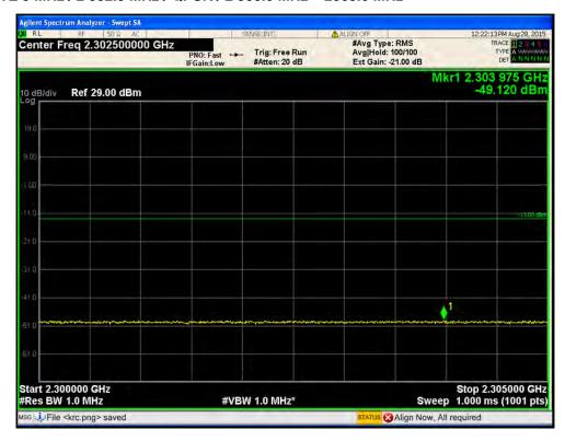
Port1 / LTE 5 MHz / 2 352.5 MHz / QPSK / 2 287.5 MHz ~ 2 300.0 MHz
