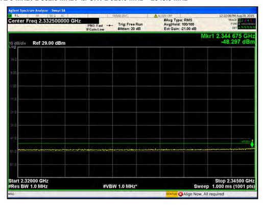
Port1 / LTE 5 MHz / 2 352.5 MHz / QPSK / 2 305.0 MHz ~ 2 320.0 MHz
