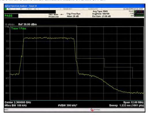
Port1 / LTE 10 MHz / 2 355 MHz / Emission Mask / QPSK / LOWER
