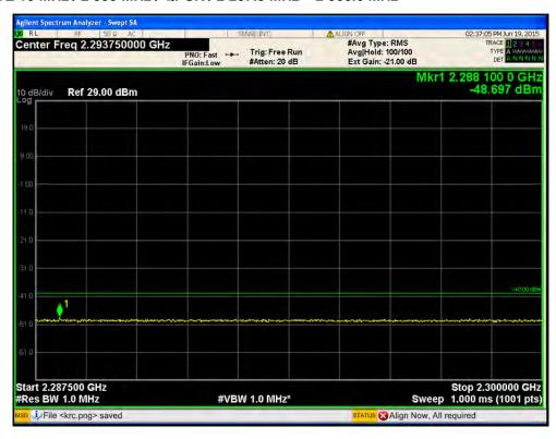
Port1 / LTE 10 MHz / 2 355 MHz / QPSK / 2 285.0 MHz ~ 2 287.5 MHz
