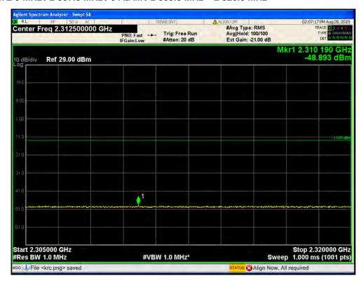
Port1 / LTE 5 MHz / 2 357.5 MHz / 64QAM / 2 300.0 MHz ~ 2305.0 MHz
