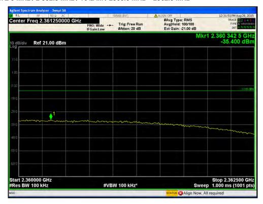
Port1 / LTE 5 MHz / 2 352.5 MHz / 16QAM / 2 362.5 MHz ~ 2365.0 MHz
