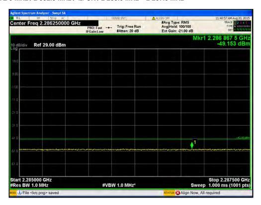
Port1 / LTE 5 MHz / 2 352.5 MHz / QPSK / below 2 285.0 MHz
