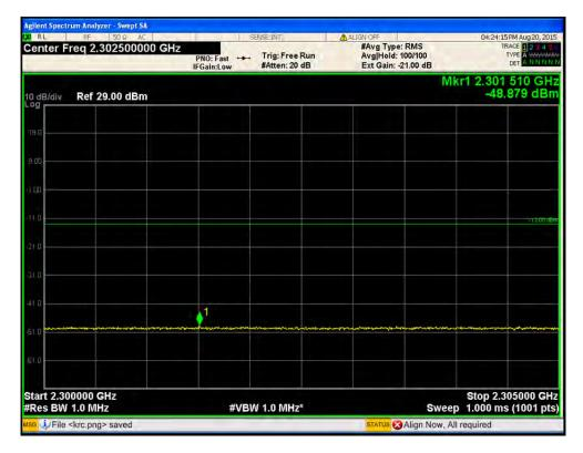
Port1 / LTE 5 MHz / 2 352.5 MHz / 64QAM / 2 287.5 MHz ~ 2 300.0 MHz
