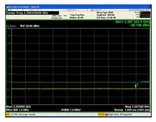
Port1 / LTE 5 MHz / 2 357.5 MHz / 64QAM / below 2 285.0 MHz
