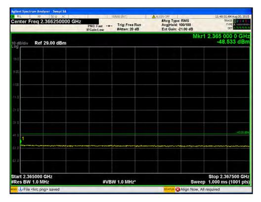
Port1 / LTE 5 MHz / 2 357.5 MHz / QPSK / 2 367.5 MHz ~ 2370.0 MHz
