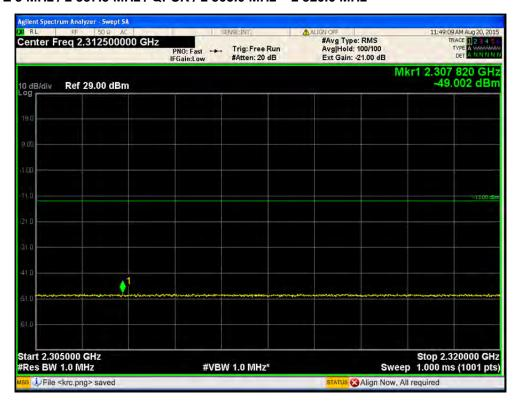
Port1 / LTE 5 MHz / 2 357.5 MHz / QPSK / 2 300.0 MHz ~ 2305.0 MHz
