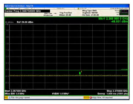
Port1 / LTE 5 MHz / 2 352.5 MHz / QPSK / above 2 370.0 MHz
