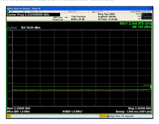
Port1 / LTE 5 MHz / 2 352.5 MHz / 64QAM / 2 305.0 MHz ~ 2 320.0 MHz
