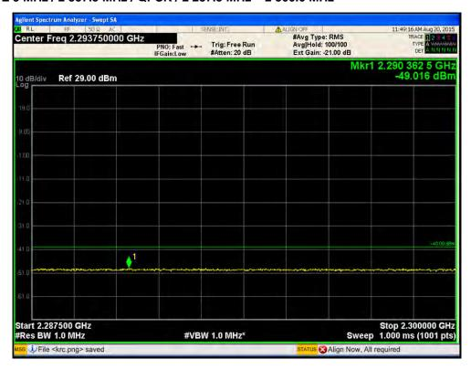
Port1 / LTE 5 MHz / 2 357.5 MHz / QPSK / 2 285.0 MHz ~ 2 287.5 MHz
