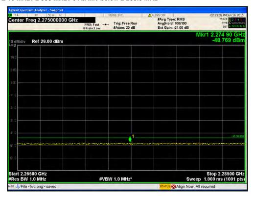
Port1 / LTE 5 MHz / 2 352.5 MHz / QPSK / 2360.0 MHz ~ 2362.5 MHz
