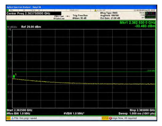
Port1 / LTE 5 MHz / 2 352.5 MHz / QPSK / 2365.0 MHz ~ 2367.5 MHz
