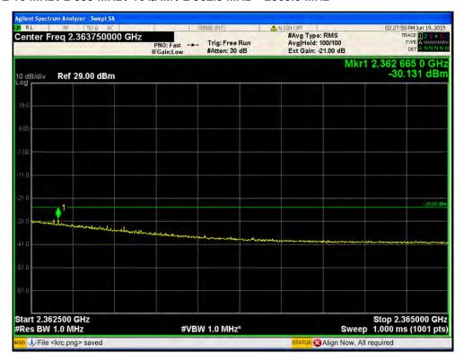
Port1 / LTE 10 MHz / 2 355 MHz / 16QAM / 2365.0 MHz ~ 2367.5 MHz
