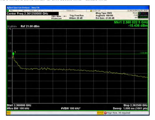
Port1 / LTE 5 MHz / 2 357.5 MHz / QPSK / 2 362.5 MHz ~ 2365.0 MHz
