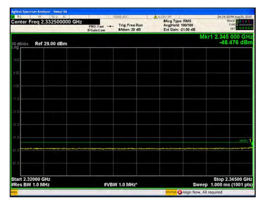
Port1 / LTE 5 MHz / 2 357.5 MHz / 64QAM / 2 305.0 MHz ~ 2 320.0 MHz
