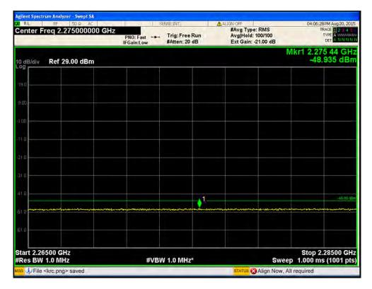
Port1 / LTE 5 MHz / 2 352.5 MHz / 64QAM / 2360.0 MHz ~ 2362.5 MHz
