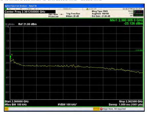
Port1 / LTE 10 MHz / 2 355 MHz / QPSK / 2 362.5 MHz ~ 2365.0 MHz
