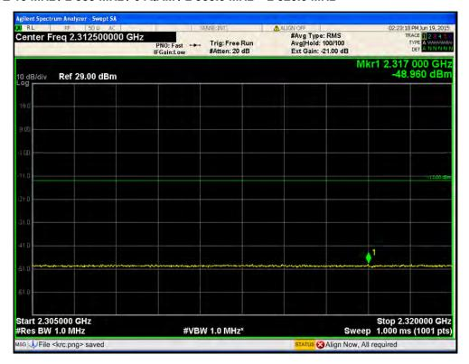
Port1 / LTE 10 MHz / 2 355 MHz / 64QAM / 2 300.0 MHz ~ 2305.0 MHz
