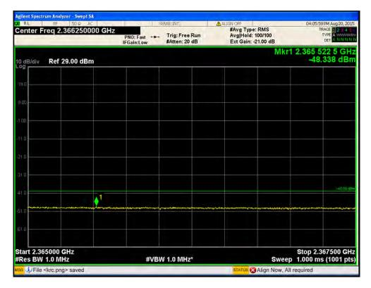
Port1 / LTE 5 MHz / 2 357.5 MHz / 16QAM / 2 367.5 MHz ~ 2370.0 MHz
