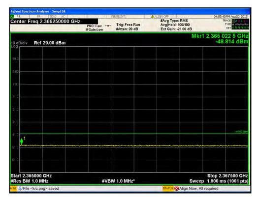
Port1 / LTE 5 MHz / 2 352.5 MHz / 16QAM / 2 367.5 MHz ~ 2370.0 MHz
