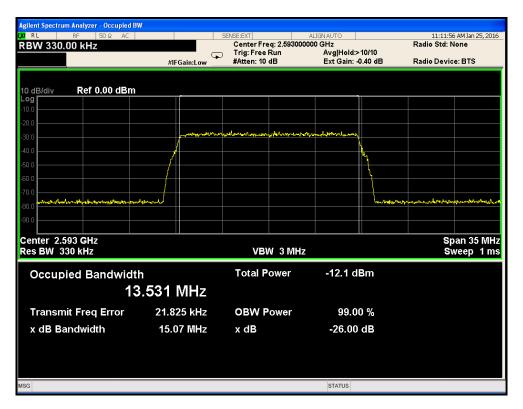
• Input signal bandwidth / 15MHz / 16QAM
