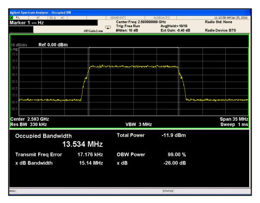
• Input signal bandwidth / 20MHz / QPSK
