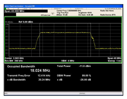
• Input signal bandwidth / 20MHz / 64QAM
