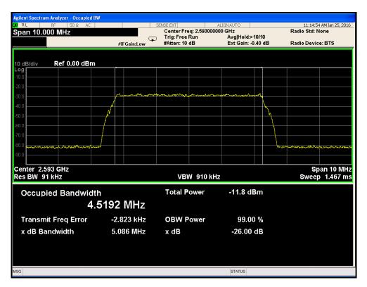
• Input signal bandwidth / 10MHz / QPSK
