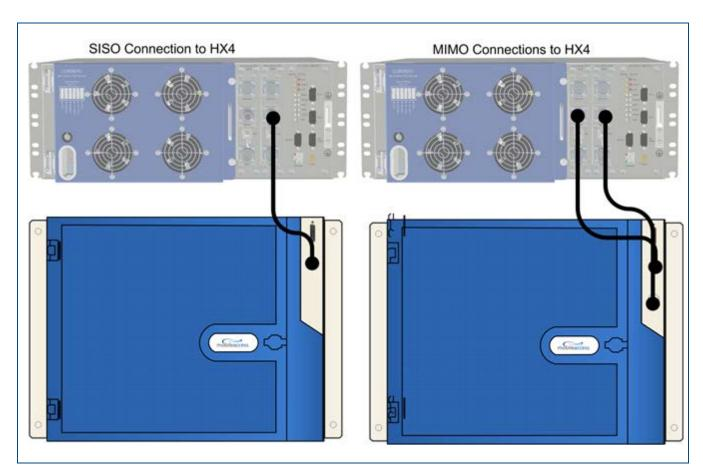
2. Connect broadband antenna coax to the HX-2.5 GHz TDD MUX module "ANT" port (two for MIMO models) and to broadband DAS antennas. Refer to Figure 3-13 for example.
