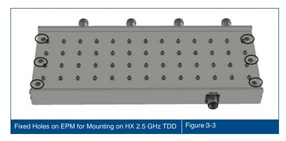
3. Place the EPM onto the top of the HX 2.5 GHz TDD unit and using six UNC 6-32, 11 mm screws (not provided), assemble the EPM onto the HX 2.5 GHz TDD unit. See Figure 3-4.
