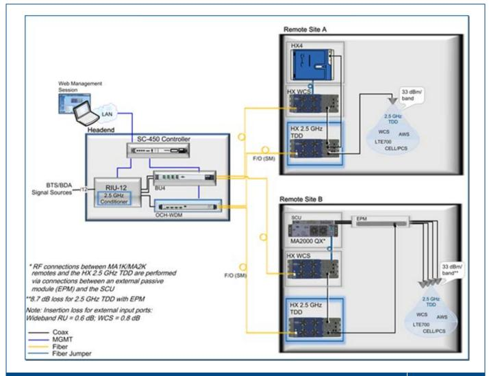
HX 2.5 GHz TDD – SISO Architecture with an existing HX4 and MA2000 QX, Sharing a Common Headend
