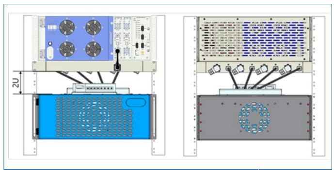
Examples of HX 2.5 GHz TDD Rack Installations with Additional MA2000 TSX Remote
