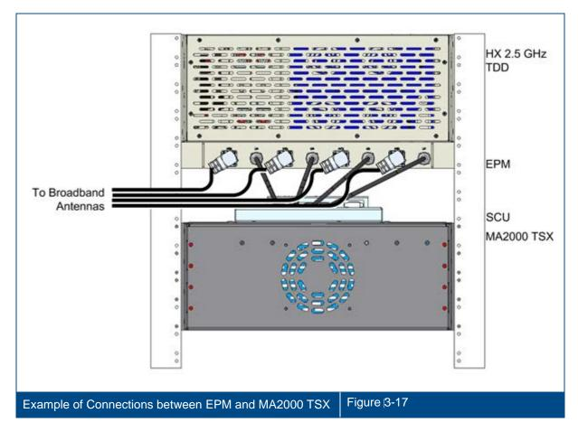
3. Connect the four EPM rear panel Mini DIN 4.3-10 "ANT" output ports to the wideband antennas.
