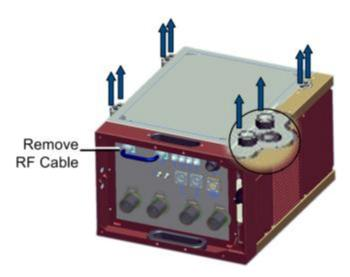
Figure 3-1. Removing GX Panel Screws
