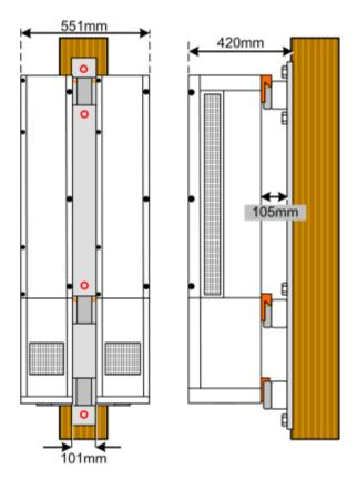
Figure 3-17. Pole Mounted GX – Dual Mount
