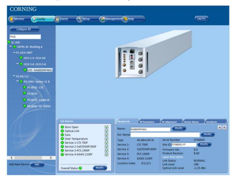
Figure 1-5. Example of GX Quad-Band Remote Configuration Tab (software v7.4)
