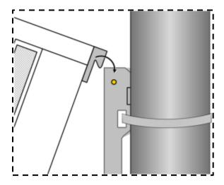
Figure 3-10. Hookiing GX to Bracket
