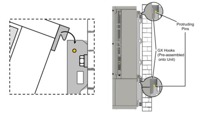
Figure 3-7. Mounting Procedure and Zoom-in of Hung Unit
