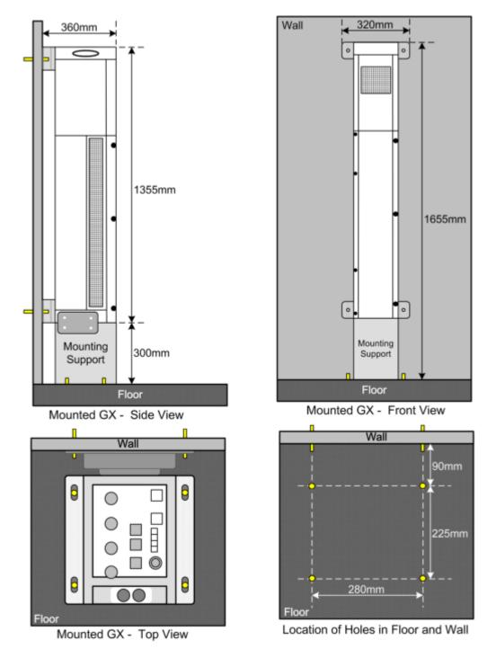
Figure 3-14. Overview of Mounting Procedure
