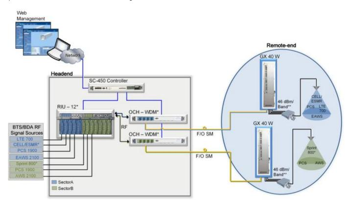
\*In installations including a GX supporting the CELL band and a GX supporting the Sprint800 band, the CELL and Sprint service signals must be conditioned via two independent sectors in the RIU-12 (i.e., SectorA and SectorB in Figure 2) and routed through dedicated optical modules in the OCH. Note the following:
