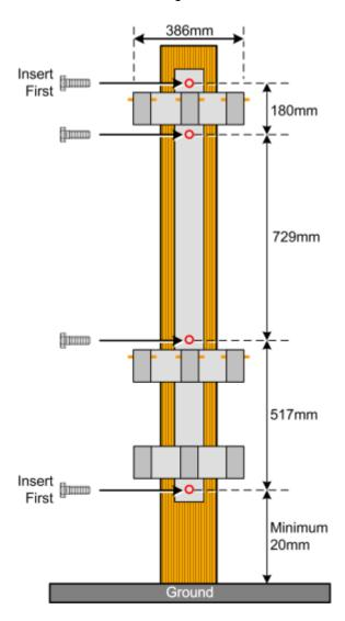
Figure 3-19. Mounting the Bracket
