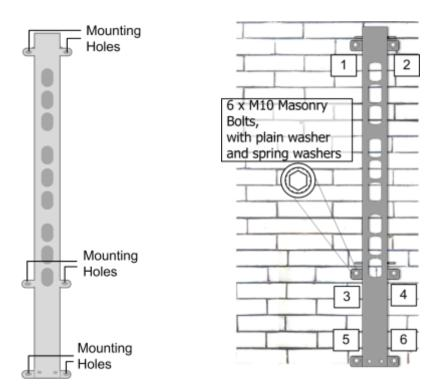
Figure 3-6. GX Mounting Bracket
