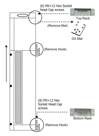
Figure 3-13.Pre-Mounting Procedure
