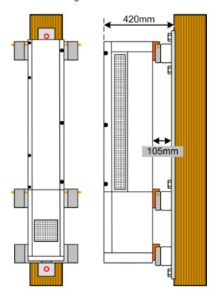
Figure 3-16. Pole Mounted GX – Single Mount
