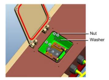
Figure 3-34. Tightening Lug to Terminal
