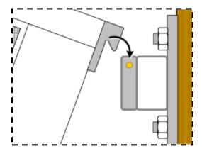
Figure 3-20. Hooking GX onto Bracket
