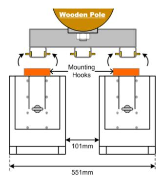
Figure 3-22. Dual GX Installation (One on each Bracket Side) - Top View
