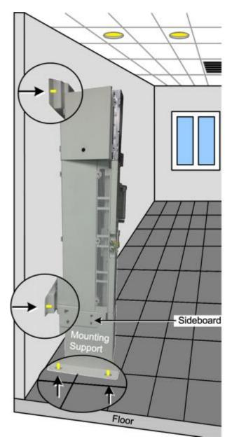
Figure 3-15.Location of Inserted Masonry Bolts
