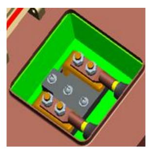
Figure 3-35. Securing Lug and Terminal
