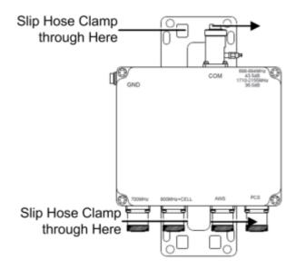
Figure 3-24. Hose Clamp Installation Holes
