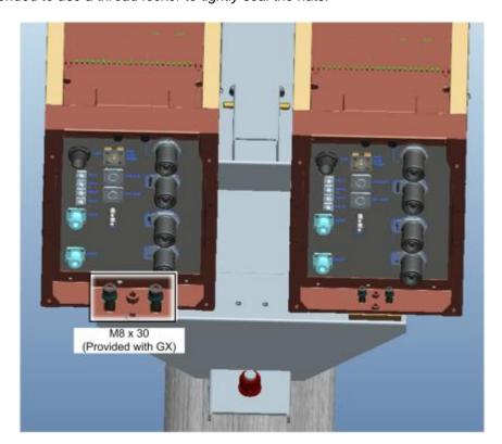
Figure 3-23. Securing GX Bottom to Bracket with M8 Screws
