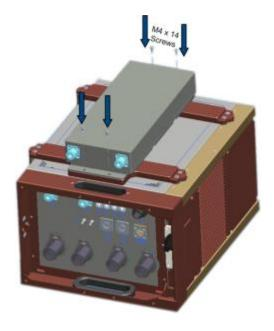
Figure 3-3. Assembling Filter onto Brackets
