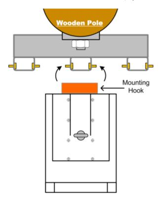
Figure 3-21. Single GX Installation (Mounted in Middle of Bracket) - Top View
