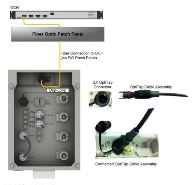
Figure 3-27. GX Fiber Optic Connection
