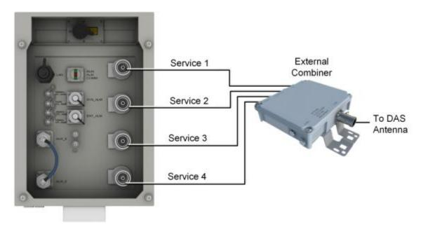
Figure 3-29. GX RF Connections with External Combiner
