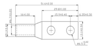
Figure 3-31. Example of Compliant DC Cable Lug
