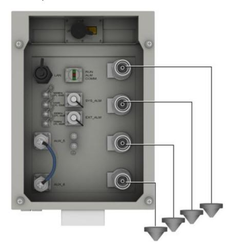
Figure 3-28. GX Direct RF Connection to DAS
