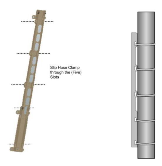
Figure 3-9. Bracket Slots for Hose Clamps (Left) and View of Bracket Mounted on Pole (Right)
