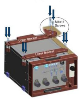
Figure 3-2. Assembling Filter Brackets
