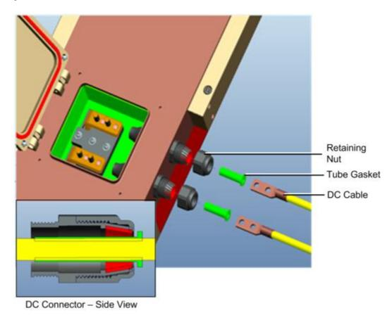
Figure 3-33. Connecting power Cord to Terminal
