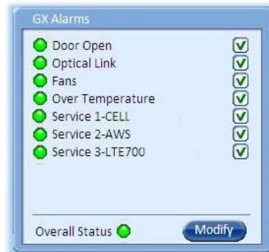
Figure 4-2: Example of GX Alarms
