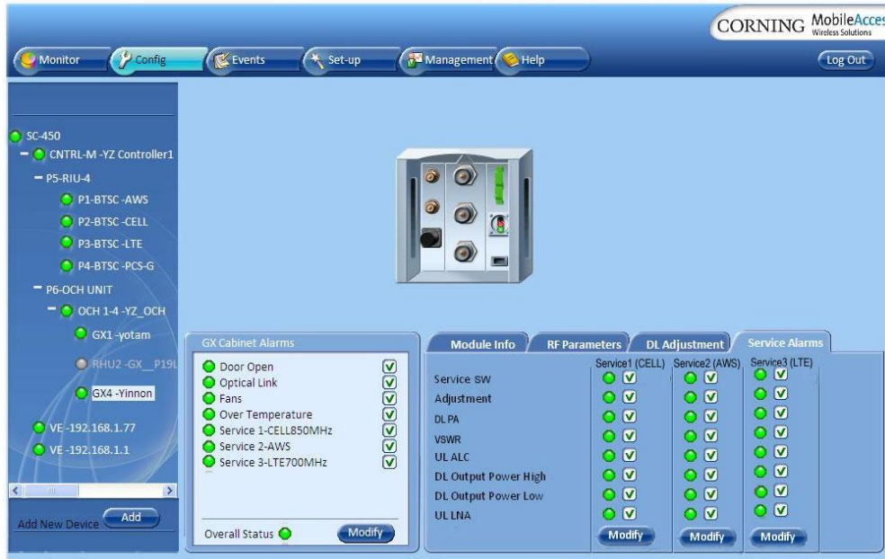
Figure 4-3. GX Service Alarms Tab
