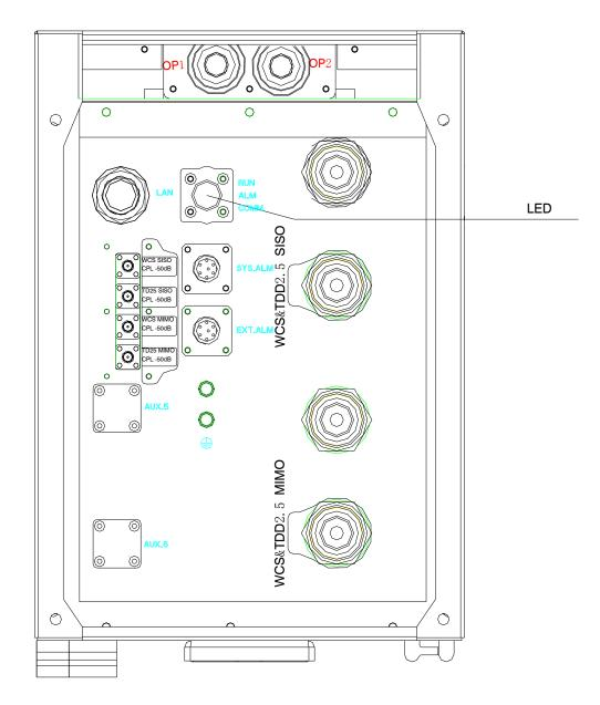
Diagnostic LEDs of each unit are located on the bottom of enclosure; each indicates the status of a particular function.
