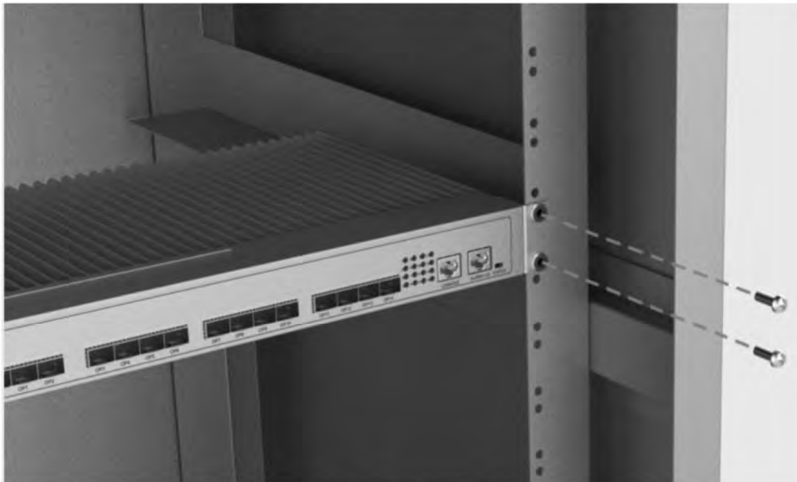
Figure 17. Place E3 in Rack
