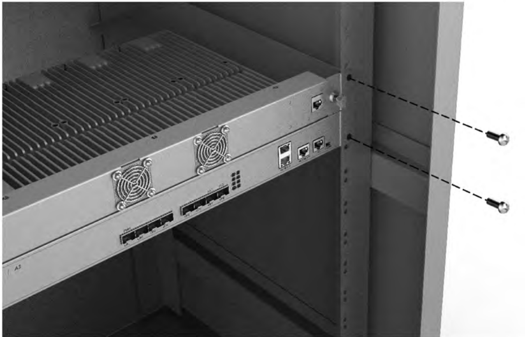
Figure 5. Place A3 in Rack
