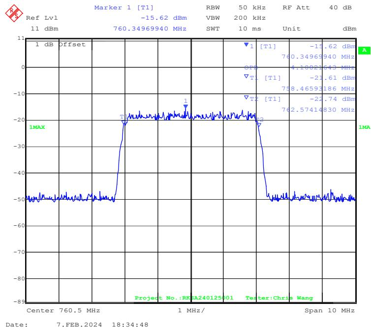
**Low Channel: 760.5 MHz, 99% Occupied Bandwidth AGC Output**
