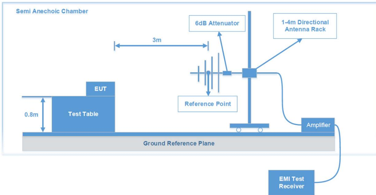
Radiated testing block diagram (above 1 GHz):
