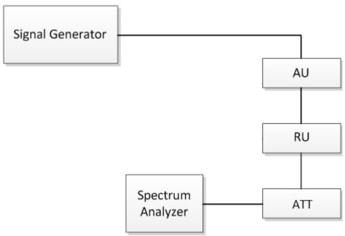
Fig.5. Out of Band rejection test configuration
