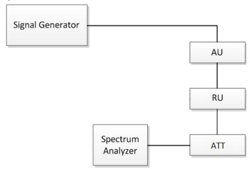
Fig.2. Conducted Spurious Emissions test configuration
