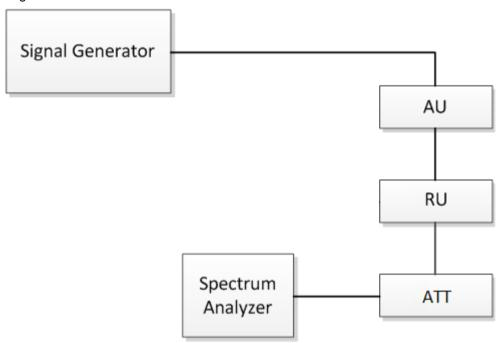
Fig.4. Occupied bandwidth test configuration
