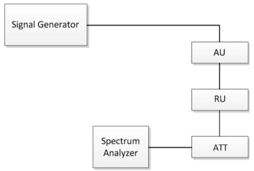
Fig.1 RF Output Power test configuration
