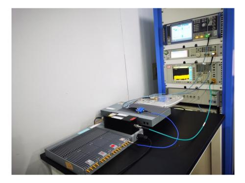
Radiated Spurious Emissions (30MHz-1GHz)
